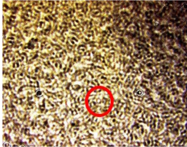
Initial Stage Top Layer Polymer at 8000x. Uniform microspheres (measurement ~0.25 microns) Uniformity and density is characteristic of polymer formation
