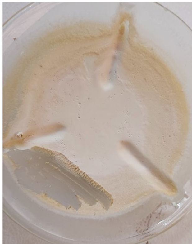
Solid form of CDB Polymer after Drying (material is pliable)
