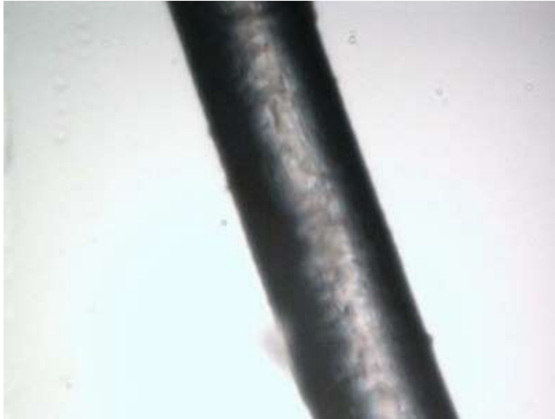
Human Hair : FOR CONTROL PURPOSES ONLY Magnification approximately 700x.. Note smooth outline and uniform size. Measurement : approximately 65 microns across. No significant internal structure or form apparent.
