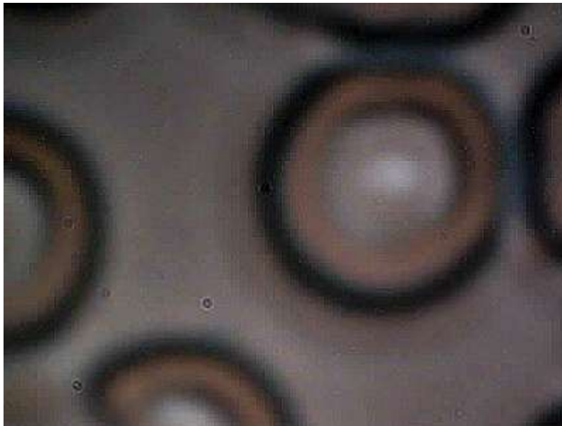
Human Hair : FOR CONTROL PURPOSES ONLY Magnification approximately 700x.. Note smooth outline and uniform size. Measurement : approximately 65 microns across. No significant internal structure or form apparent.
