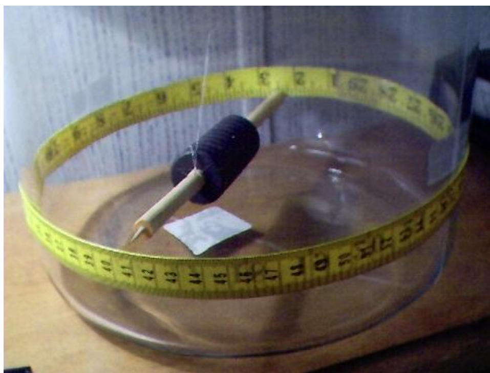
Photograph of the suspended dowel, pointer unit, dowel, magnets and graduated scale.
