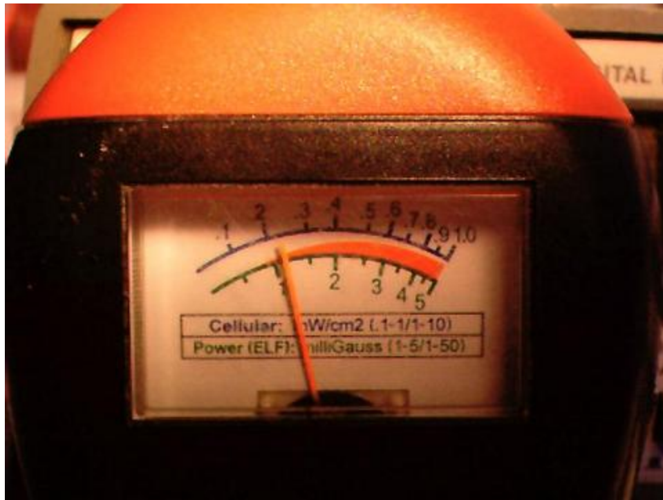
Photos which show stages of oscillation of the needle in response to a resonant frequency. (1 of 2)
