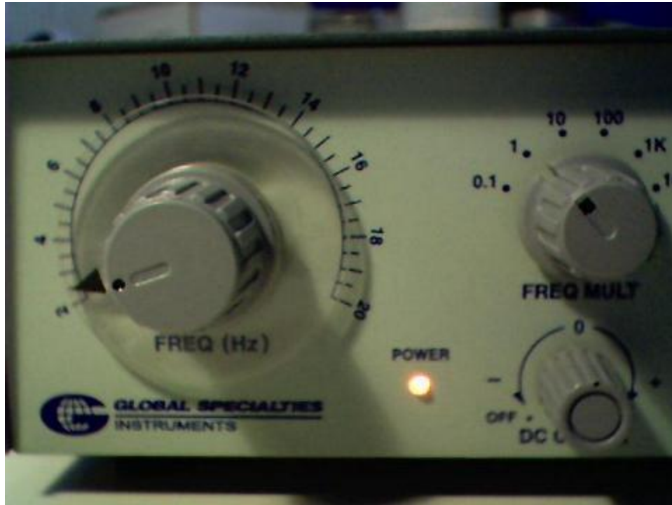
Sine wave generator used to introduce a signal into the circuit.
