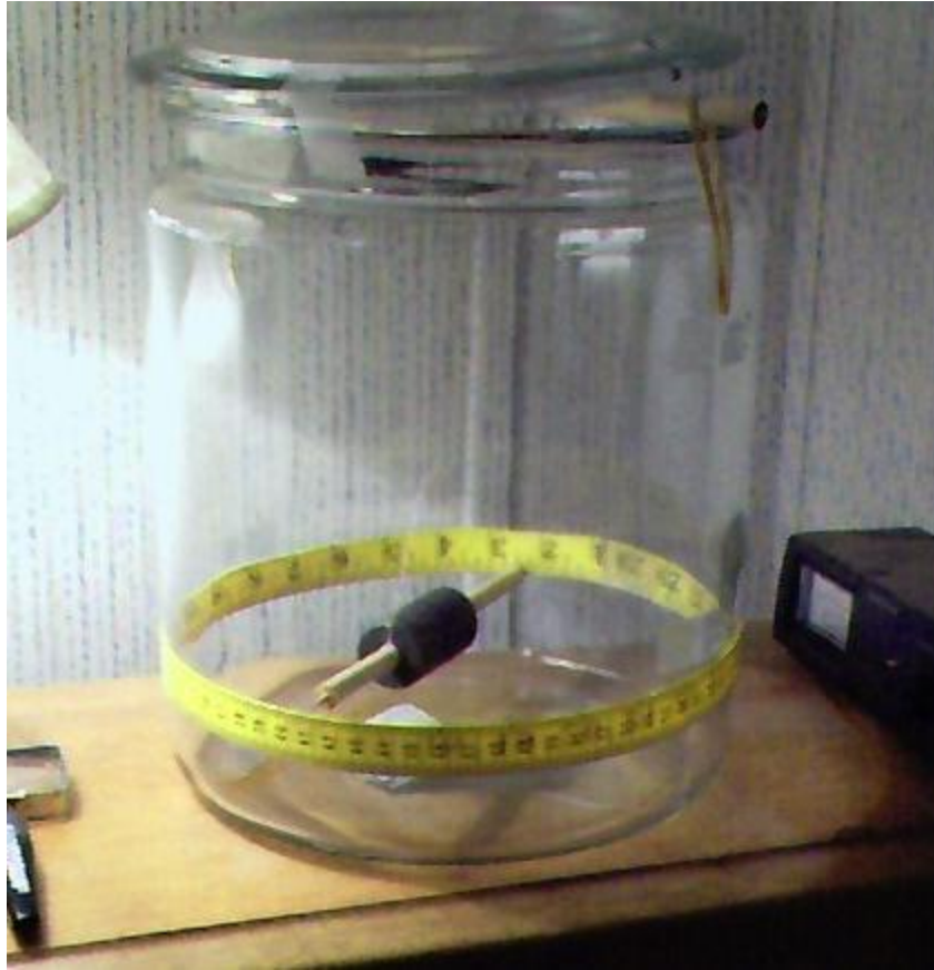
Photograph of the Magnetometer, showing glass housing unit, suspended dowel with 10 ring magnets, and graduated scale.
