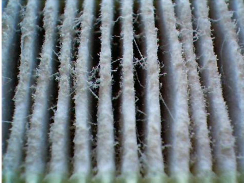
HEPA Filter in residential service(indoor) for approximately 3 weeks.
